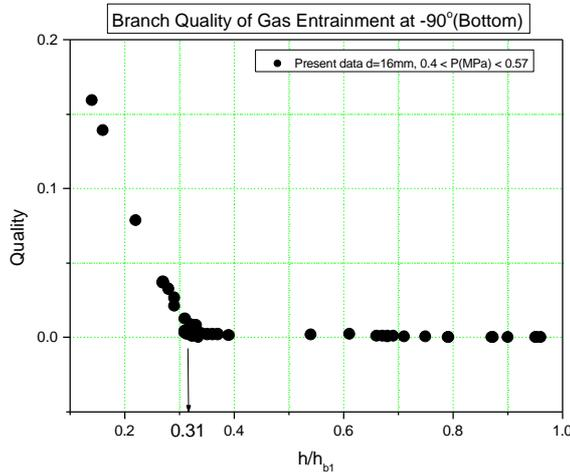
Figure 8 Quality data for the new onset definition at bottom branch
