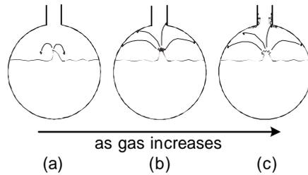
Figure 3 Development of liquid entrainment at the top branch
