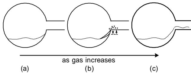
Figure 4 Development of liquid entrainment at the side branch
