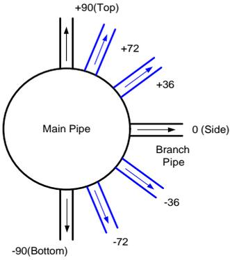
Figure 2 Side view of T-junctions
