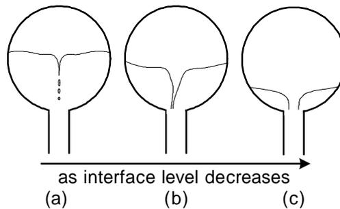
Figure 6 Development of gas entrainment at the bottom branch
