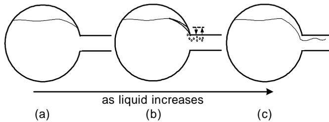
Figure 5 Development of gas entrainment at the side branch
