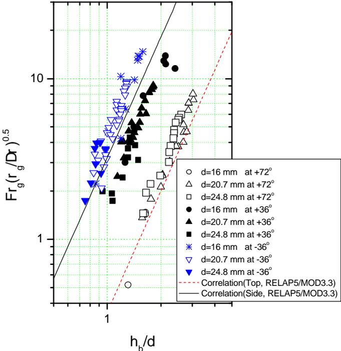
Figure 11 Comparison of the O.L.E. data at  $+72^\circ$ ,  $\pm 36^\circ$  branches
