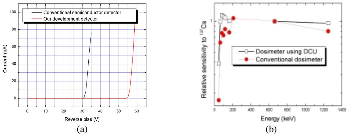
Figure. 6 (a) Electronic analysis and (b) comparison of the relative energy sensitivity to Cs-137 using the conventional method and that using dose conversion algorithm.
