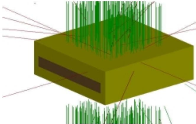
Figure. 1. Monte Carlo simulation geometry of silicon PIN photodiode for filter design.
