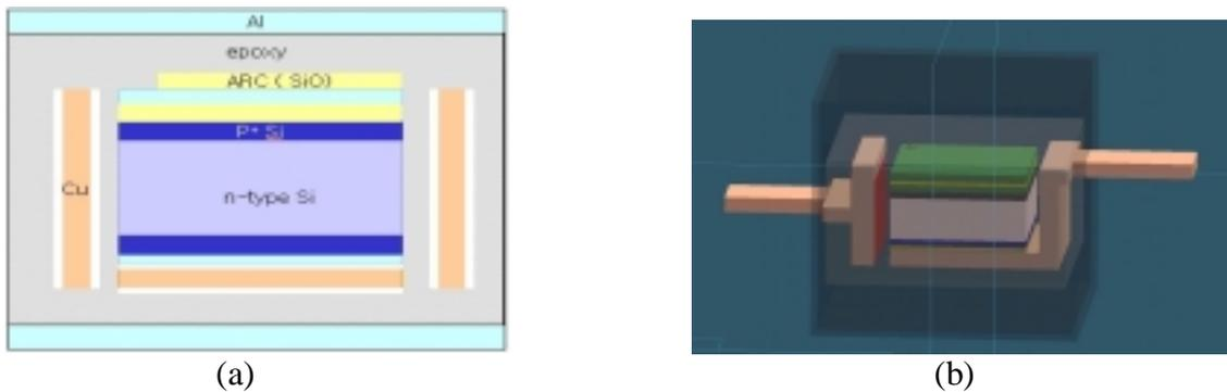
Figure. 2. (a) A schematic geometry of PIN detector and (b) the designed dosimeter.
