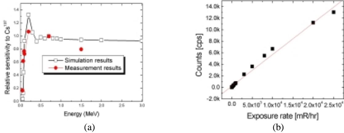
Figure. 5 (a) Comparison of relative energy sensitivities between MCNP simulations and measurements with KAERI x-ray beam and gamma source and (b) counts rate due to the variation of exposure dose rate.
