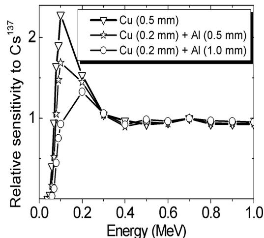
Figure. 4 Relative energy sensitivity to Cs-137 due to change of filter thickness and materials.
