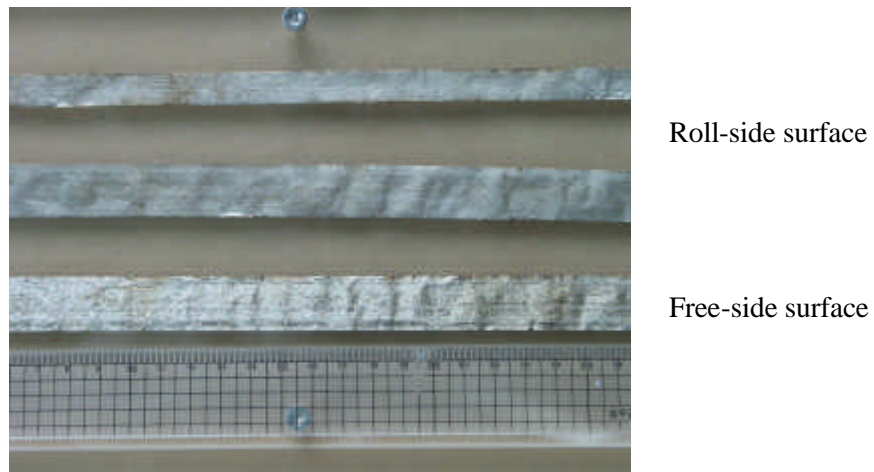
Fig. 2. Continuous uranium foils produced by cooling-roll casting apparatus.
