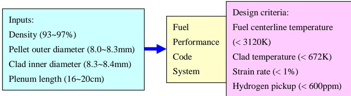
Figure 14. Configuration of optimization method for fuel design parameters.
