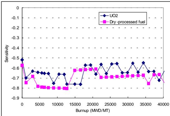
Fig. 3. Sensitivity of fuel centerline temperature for fuel density.
