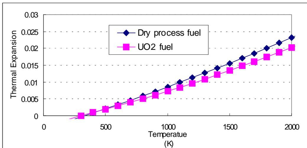
Figure 2. Thermal expansion for dry process fuel and UO<sub>2</sub> fuel.
