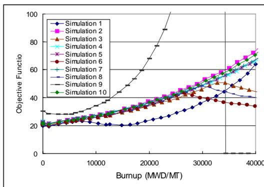
Fig. 15. Simulation of random sampling for  $UO_2$  fuel rod.
