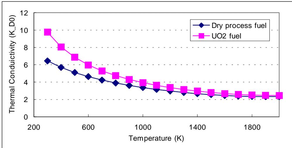
Figure 1. Thermal conductivity for dry process fuel and UO<sub>2</sub> fuel.
