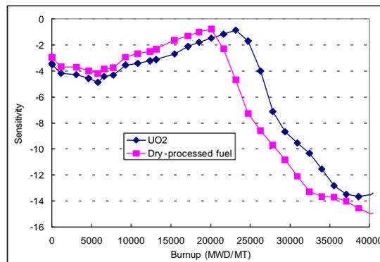
Fig. 8. Sensitivity of internal pressure for cladding inner diameter.
