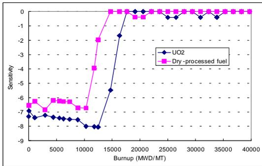
Fig. 9. Sensitivity of fuel centerline temperature for pellet outer diameter.
