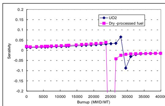
Figure 13. Sensitivity of internal pressure for plenum length.
