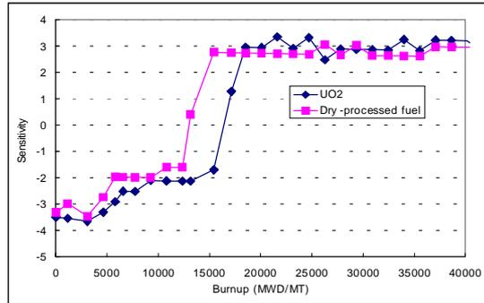
Fig. 6. Sensitivity of fuel centerline temperature for cladding inner diameter.
