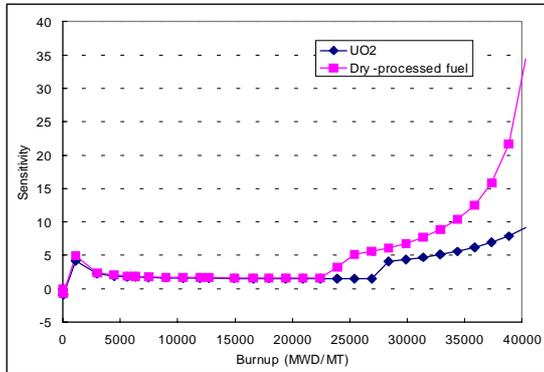
Fig. 4. Sensitivity of strain for fuel density.
