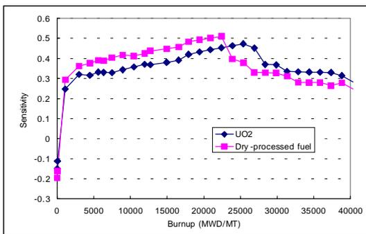
Fig. 5. Sensitivity of internal pressure for fuel density.
