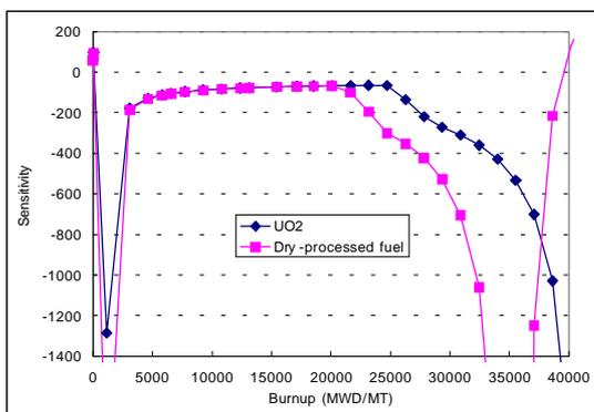
Fig. 7. Sensitivity of strain for cladding inner diameter.
