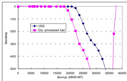
Fig. 10. Sensitivity of strain for pellet outer diameter.
