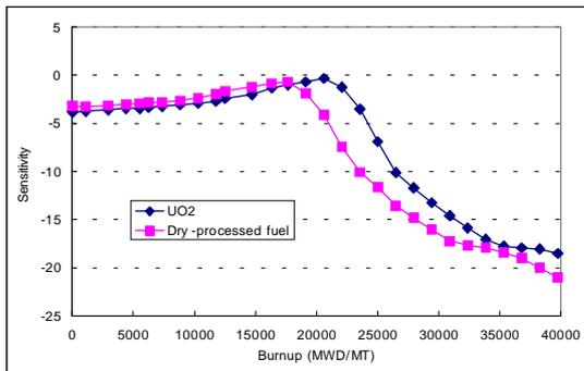
Fig. 11. Sensitivity of internal pressure for pellet outer diameter.
