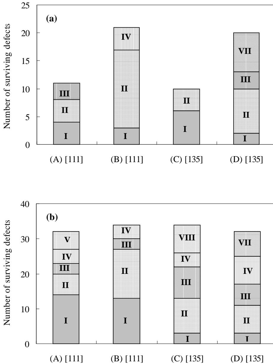
Figure 3. Interstitial cluster spectrum for  $\alpha$ -iron at 290°C at the end of an MD simulation. Roman numerals inside the box stand for the size of interstitial clusters (I : single interstitial, II : di-interstitial, III : tri-interstitial, etc.). The number in the bracket on the abscissa is the initial direction of PKA. (a) 2 keV Iron cascade and (b) 4 keV Iron cascade.
