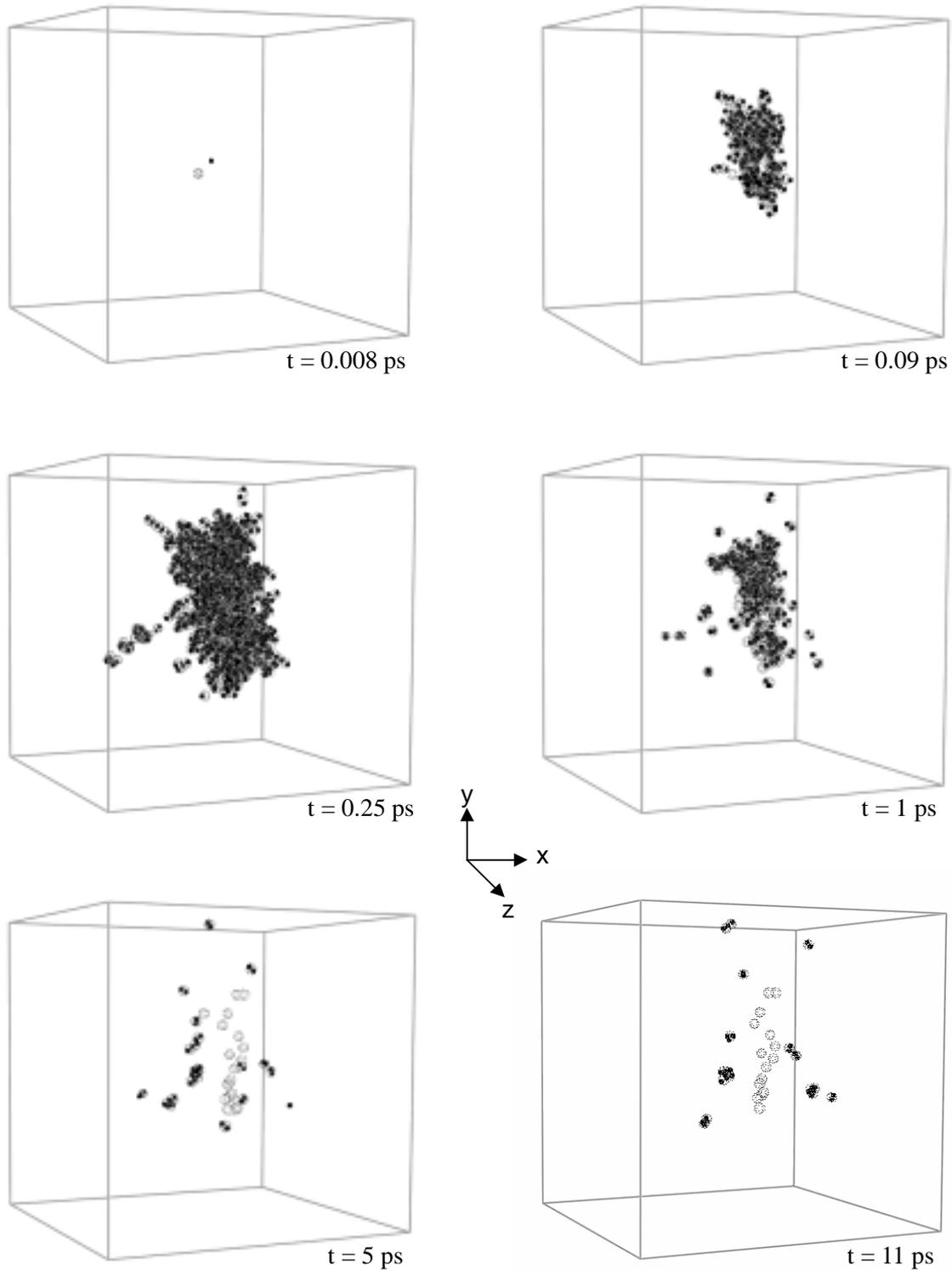
Figure 1. Illustration of displacement cascade evolution from a 4 keV PKA simulation in  $\alpha$ -iron at 290°C. The size of the atomic block is  $40a_0 \times 40a_0 \times 40a_0$  ( $a_0$ : lattice constant) and the initial PKA direction [135]. Filled squares represent interstitial atoms and empty ones vacancies
