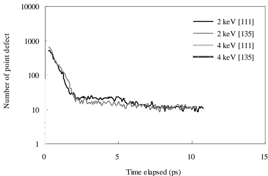
Figure 2. Variation of the number of point defects with time elapsed for four cascades at 290°C. The simulation PKA energies are 2 and 4 keV with different initial PKA directions of [111] and [135].
