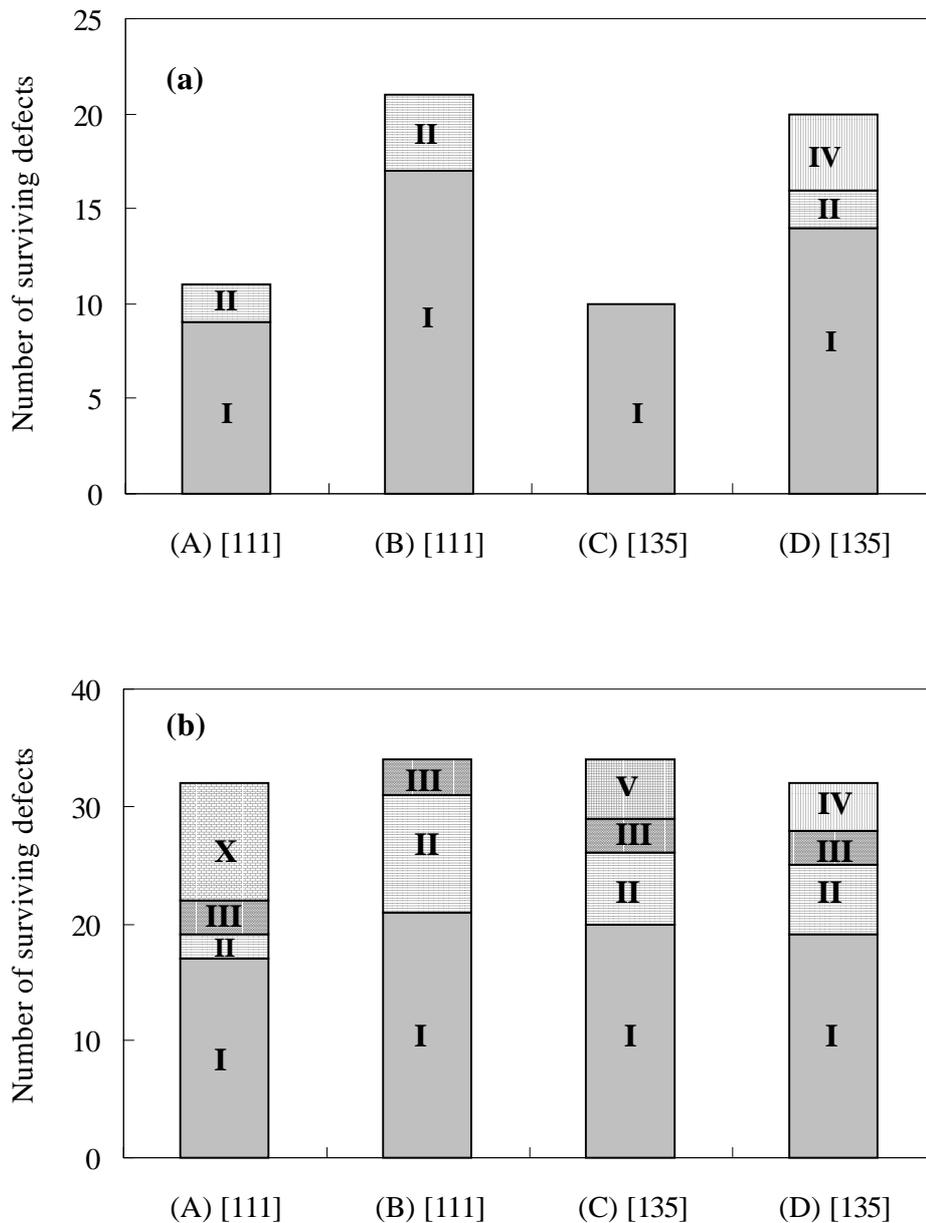
Figure 4. Vacancy cluster spectrum for  $\alpha$ -iron at 290°C at the end of an MD simulation. (a) 2 keV Iron cascade and (b) 4 keV Iron cascade.
