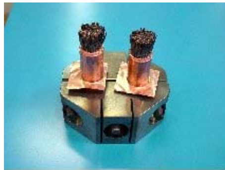
Fig. 3 Two CICC specimens are assembled by low carbon steel clamp.
