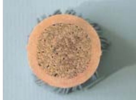
Fig. 1 Cross section of the compacted cable ( V_f :15%).
