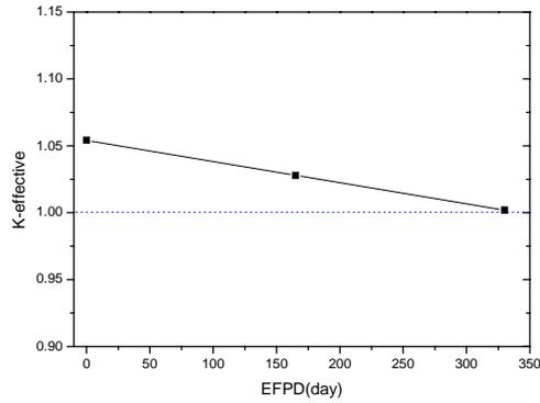
Fig. 1. Excess reactivity change of PEACER core
