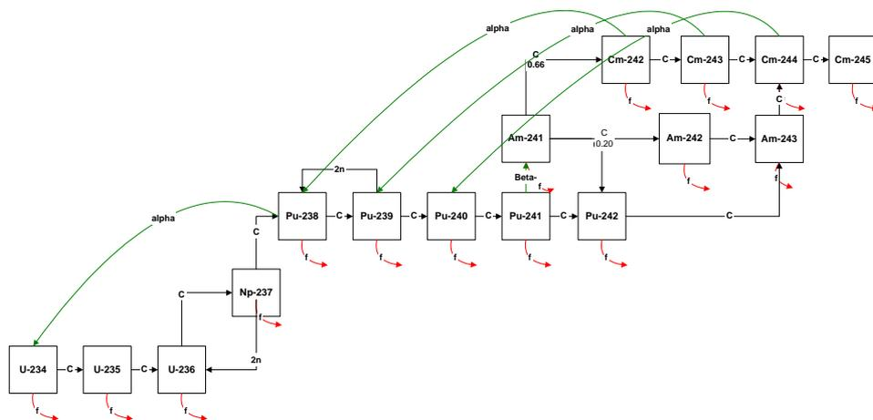
Fig. 3. User defined depletion chain for REBUS-3 calculation and transmutation indices
