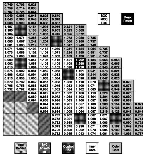
Fig. 2. Assembly power distribution in equilibrium state
