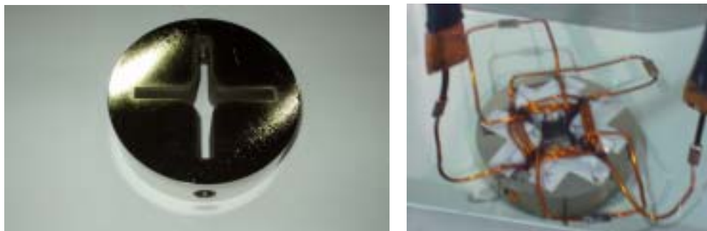
Figure 10. (a) Fabricated iron core sample and (b) coil test
