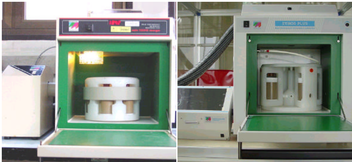
Fig. 1. Closed vessel acid digestion system. (Milestone MLS1200 and Ethos Plus)
