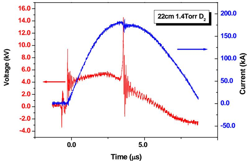
Figure 6. Voltage spike and Current drop signal measured in DPF-device
