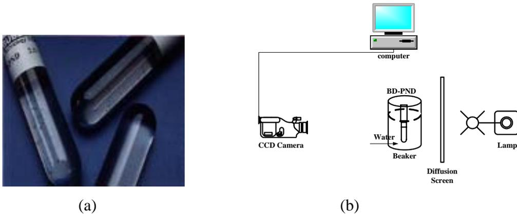
Figure 2. (a) Neutron Bubble Dosimeter (BD-PND: Bubble Technology Industry),
