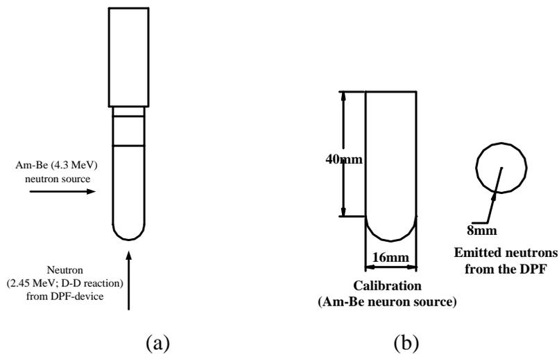
Figure 3. (a) Irradiated neutron direction for the BD-PND,
