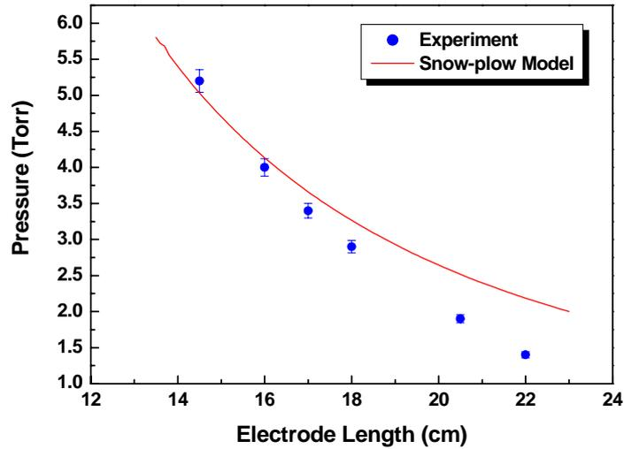
Figure 5. Optimum deuterium filling pressure for different electrode lengths
