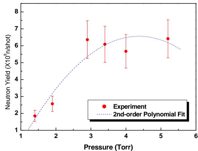
Figure 8. Dependence of the average neutron yield with the deuterium filling pressure
