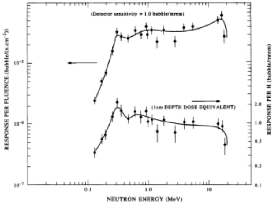
Figure 4. Neutron response curve for BD-PND
