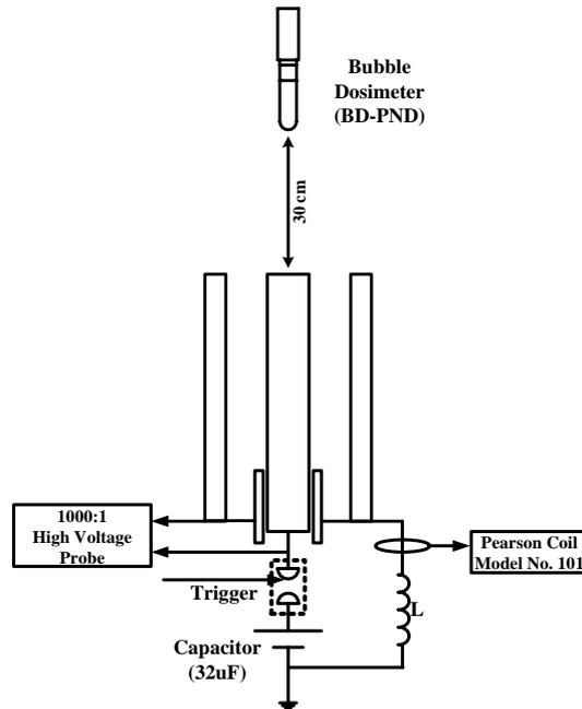
Figure 1. Schematic diagram of the DPF-device
