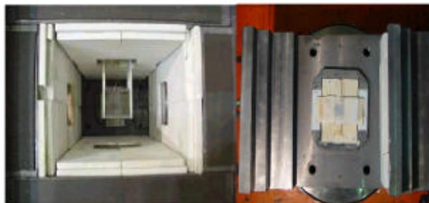
Fig. 2. Sample device and  ${}^6\text{LiF}$  tile on the beam shutter
