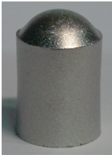
Fig. 4. Zr-U alloy sintered at 1500°C in high vacuum for 2 hours.
