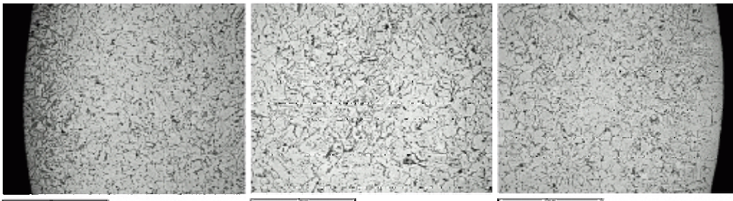
Fig. 11. SEM images of transverse section of Zr-U alloy sintered at 1500°C for 3 hours.
