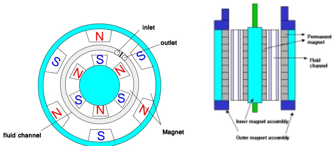
Fig. 2 Cross sectional view of separator (top & side)
