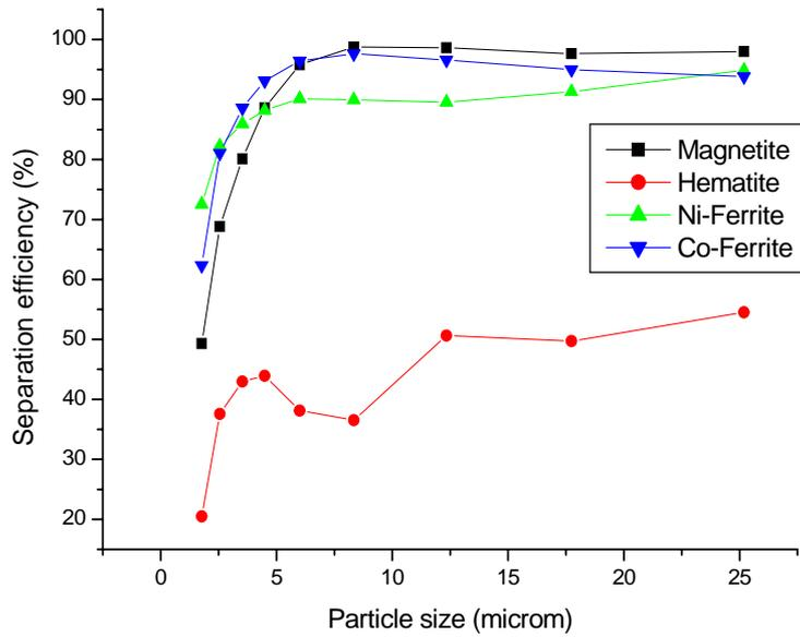
**Fig. 6 Separation efficiency as particle size (four input material, 50rpm, 0.9gpm)**
