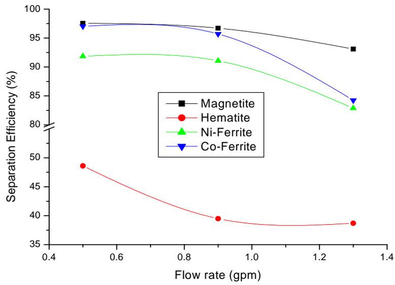
**Fig. 5 Separation efficiency at same condition ( 50rpm)**
