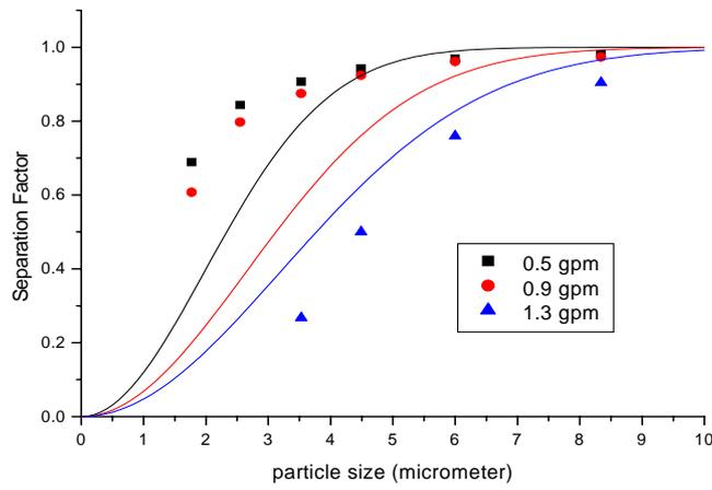
**Fig.8 Theoretical results vs experimental results (Co-ferrite, 3000Gauss)**
