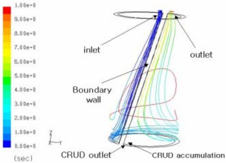
Fig. 10 Flow in the fluid channel (1gal/min)
