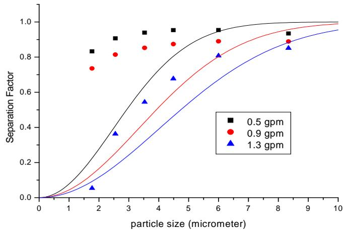
**Fig.9 Theoretical results vs experimental results (Ni-ferrite, 3000Gauss)**
