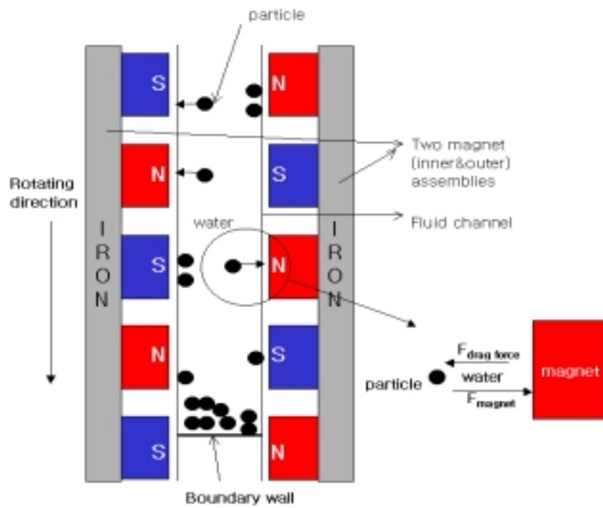
Fig. 1 Modeling of the magnetic separation of this filter
