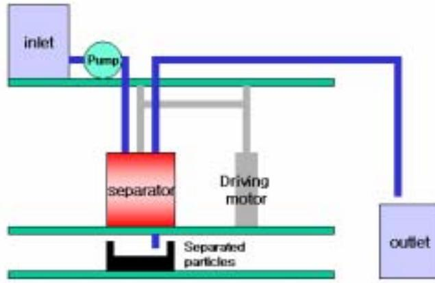
**Fig. 3** Schematic drawing of magnetic filtering system
