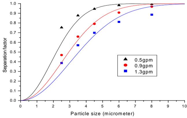
**Fig.7 Theoretical results vs experimental results (magnetite, 3000Gauss)**
