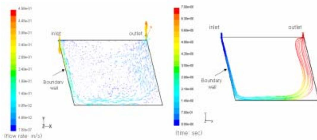
Fig. 11 Flow in the fluid channel (0.5gpm)
