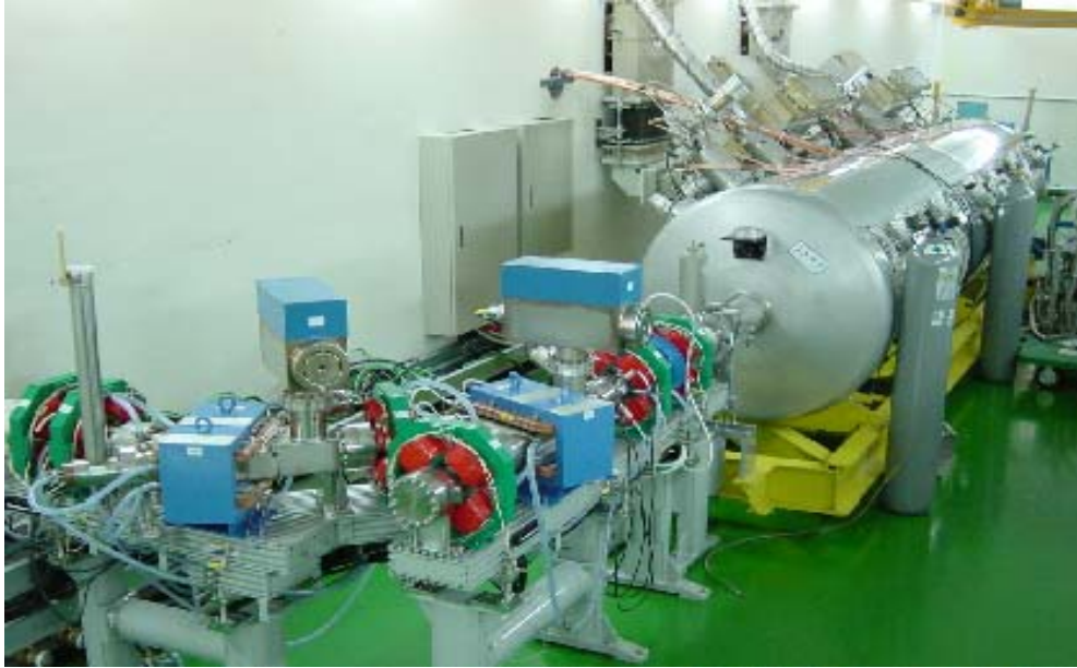
Figure 3. Photograph of the 352-MHz superconducting acceleration cavity.
