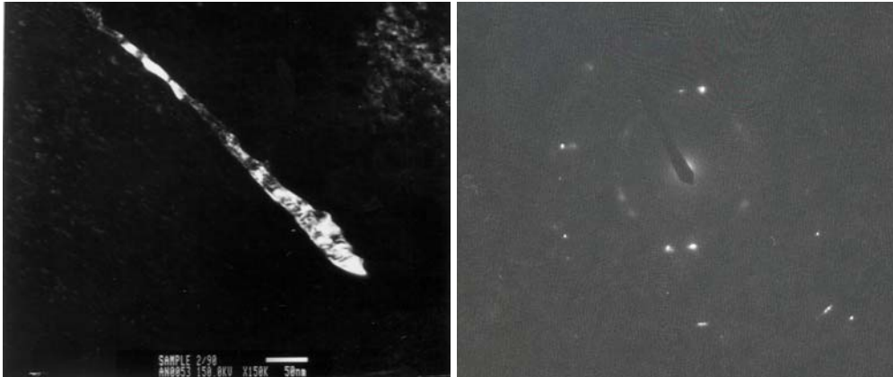
Fig. 8. Dark field image of the \beta -Zr grains in the irradiated W1 Zr-2.5Nb tube and their selected area diffraction patterns.
