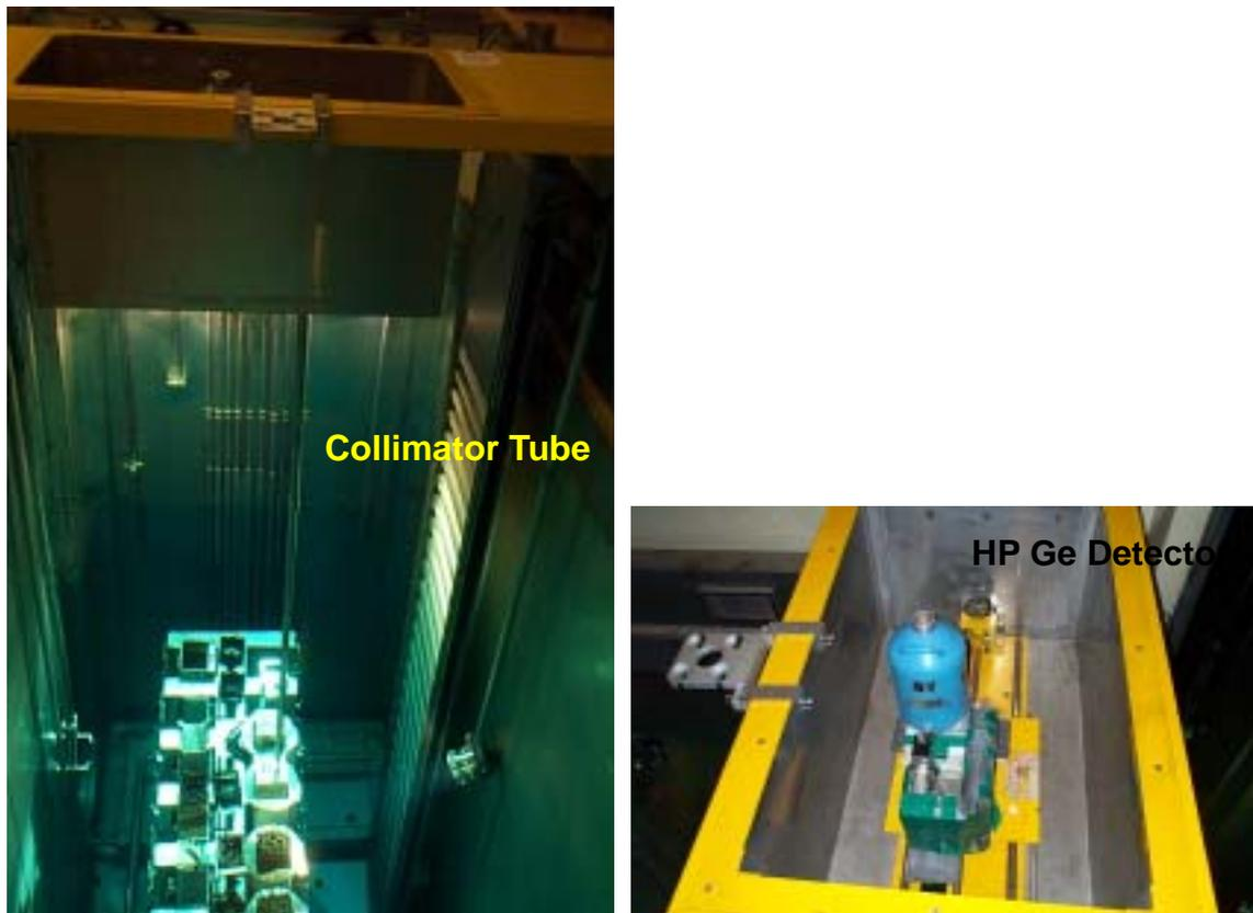
Figure 8. In-pool fuel rod verification system at KAERI
