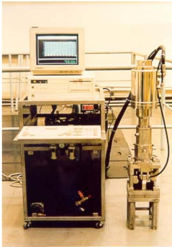
**Figure 9. In-pool Hold-down Spring Force Measuring Equipment**
