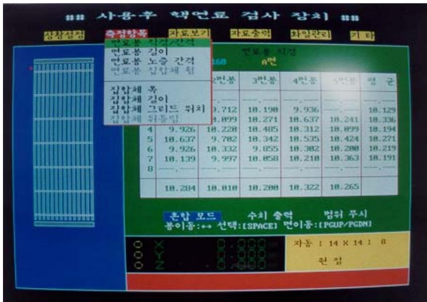
Fig. 5. Control Panel, Display Monitor & Data Acquisition System of VDIS
