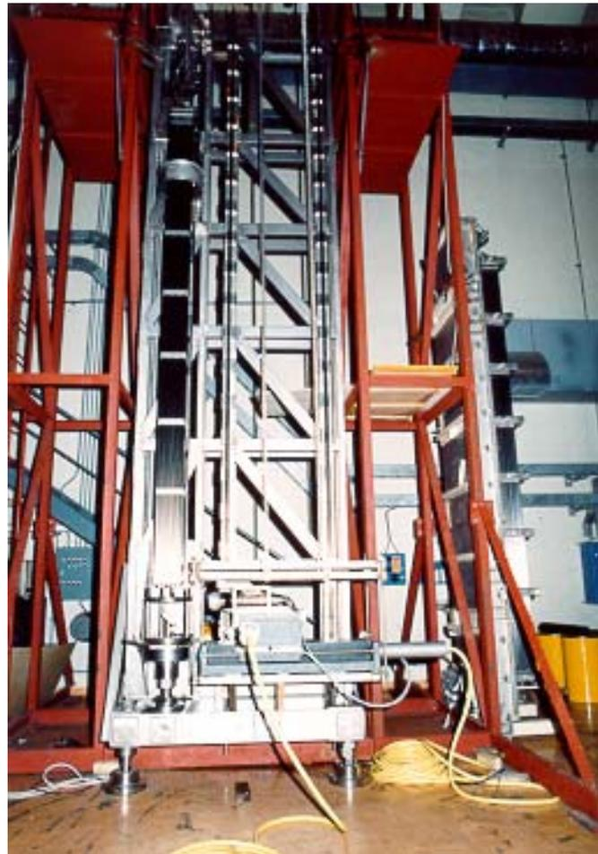
**Figure 3. A Comprehensive Transportable On-site Fuel Inspection System**
