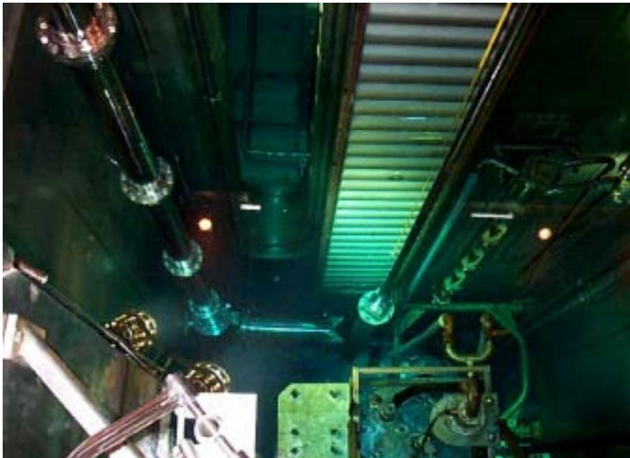
**Figure 10. Underwater Gamma Scanning System for Burnup Measurement**
