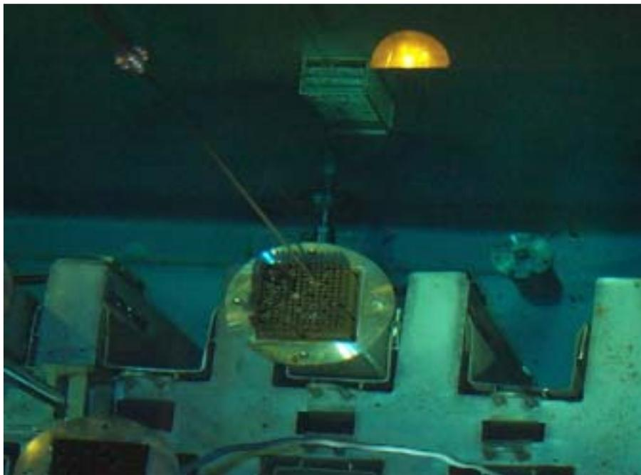
Figure 12. Exponential Experiment for Spent Fuel Assembly in PIEF Pool
