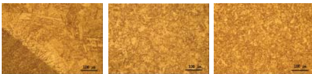
Fig. 8 Microstructural transition in the weld heat affected zone(heat input, 3.2 kJ/mm, x200). (a) Grain-coarsened region adjacent to fusion line, (b) intermediate grain-refined region and (c) grain-refined region.
