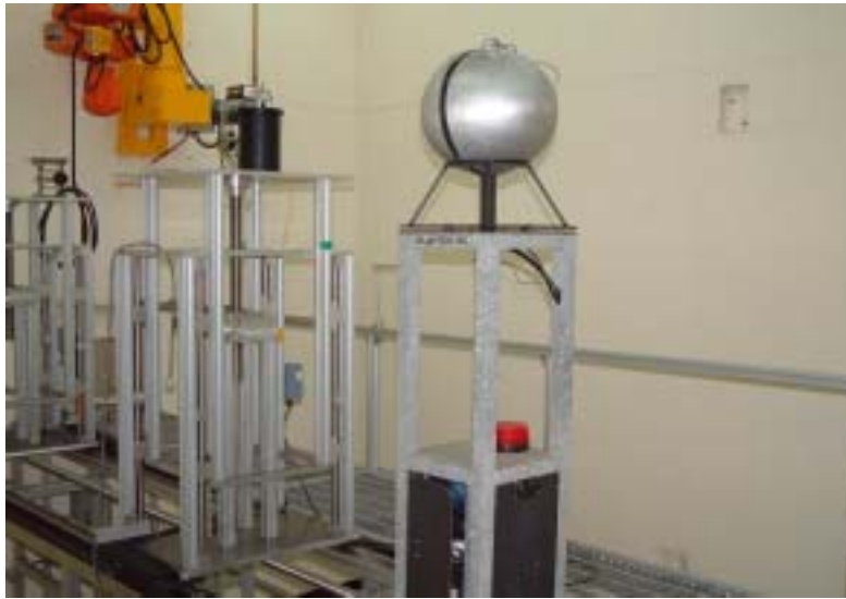
Fig. 2. Neutron source ^{252}\text{Cf} Neutron source of KAERI (with \text{D}_2\text{O} moderator of 30cm )
