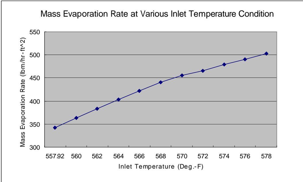
Figure 4.  $\dot{M}_e$  at Various Inlet Temperature Condition for Kori Units 3&4
