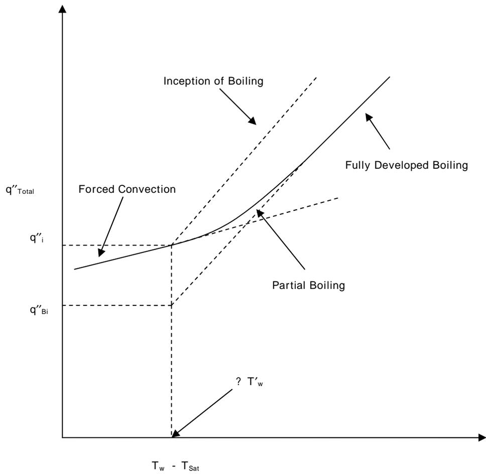
Figure 1. Bergles and Rohsenow Boiling Model
