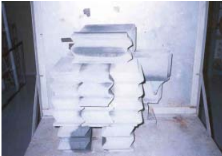
Fig. 7. Arrangement of Block for Exclusion of Scattering Radiation
