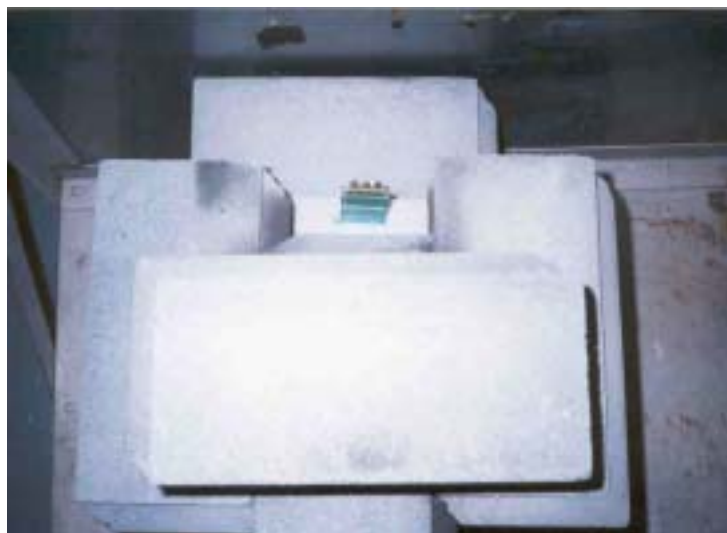
Fig. 6. Ceric-cerous Surface Dosimeter for Measurement of Dose Rate.
