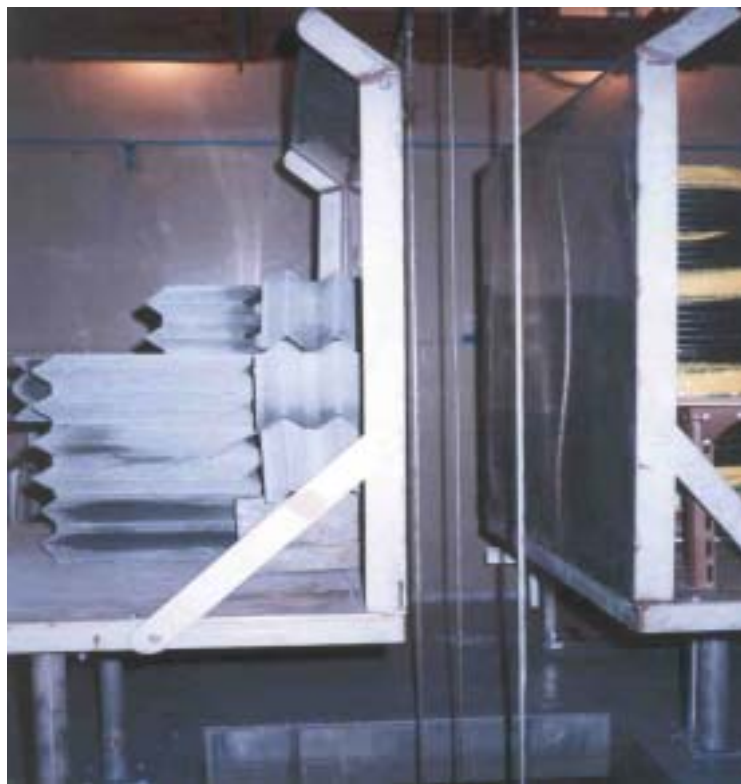
Fig. 8. Loading System of Co-60 Plate Source.
