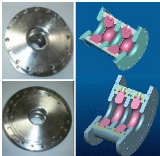
Photo 1. Fabricated Einzel lenses. Right side shows the cross sectional desing of the lenses.
