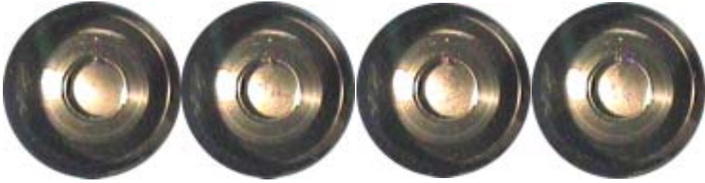
Fig. 9 Bubble float at 6\mu\text{A} proton beam irradiation (0.25sec interval)
