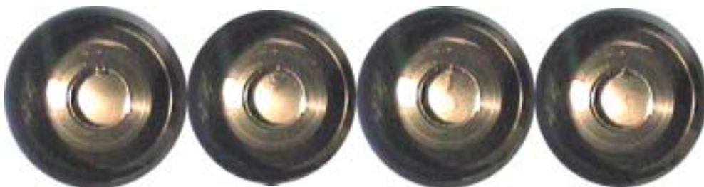
Fig. 8 Bubble float at 5μA proton beam irradiation (0.25sec interval)
