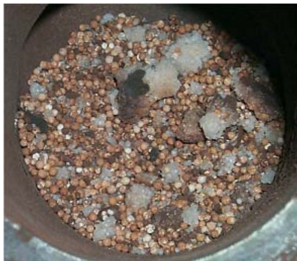
Fig. 4. The photograph of SLZ after reaction( r=1.0 , \text{LiCl}+\text{CsCl}+\text{SrCl}_2 , Zeolite 4A bead, 500\text{ }^\circ\text{C} , 17\text{ rpm} ).
