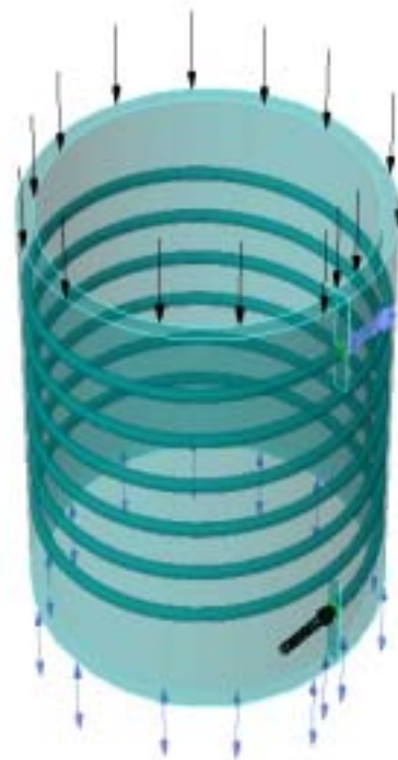
Figure 2. Helical coiled tube model for CFD analysis
