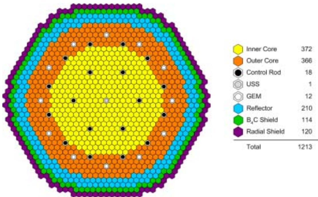
Fig. 2. Radial Configuration of the Modified BN-600 Core (Case 2)
