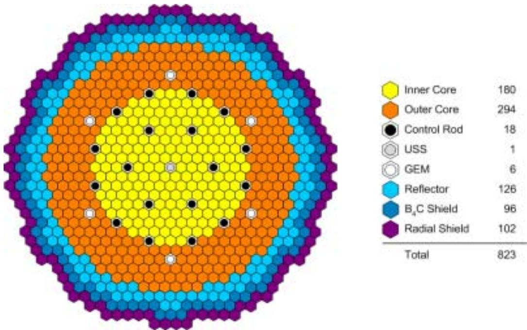
Fig. 1. Radial Configuration of the Modified BN-600 Hybrid Core (Case 1)
