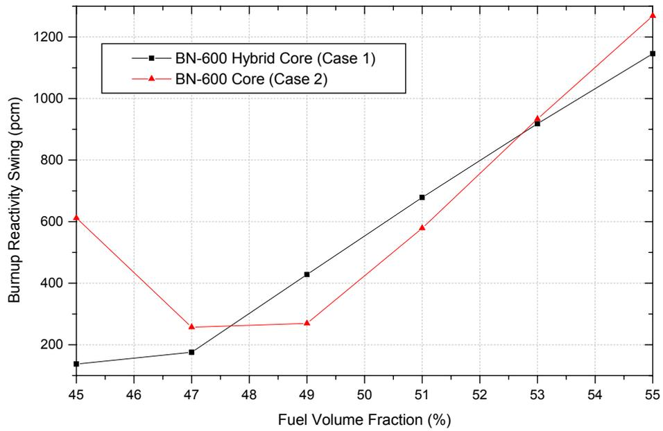
Fig. 4. Burnup Reactivity Swing vs. Fuel Volume Fraction
