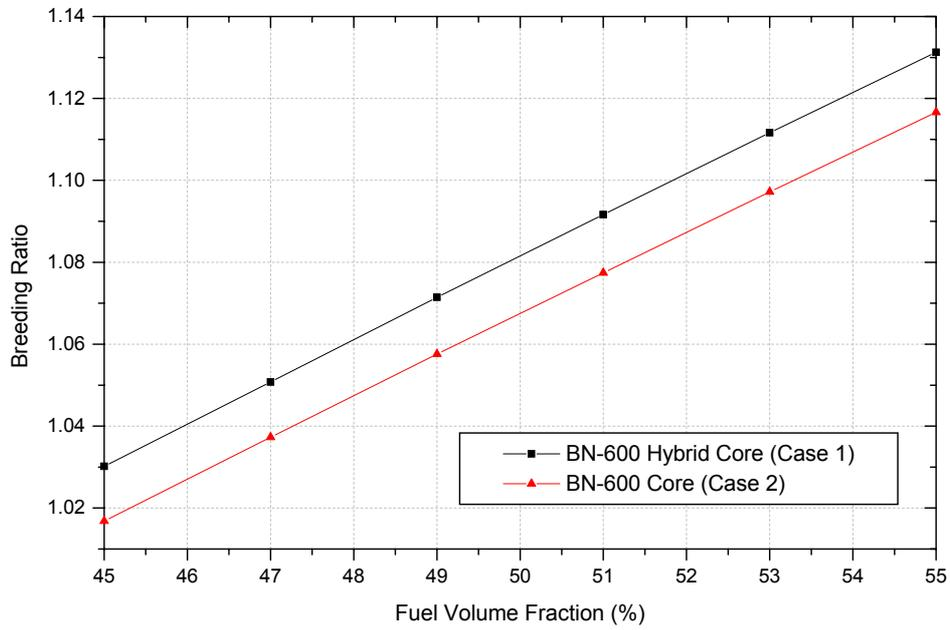
Fig. 3. Breeding Ratio vs. Fuel Volume Fraction
