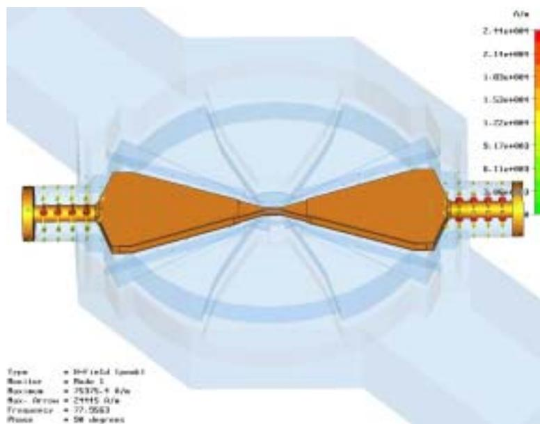
Figure 3: Magnetic field distribution
