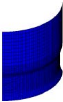
Cycle 5 (X 2) Thermal Ratcheting
