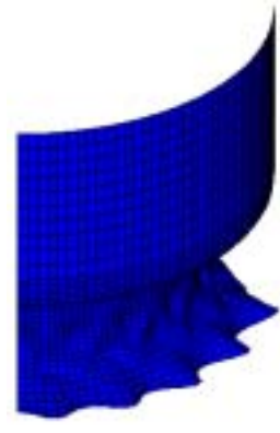
Cycle 15 (X 5) Buckling All Moving Zone
