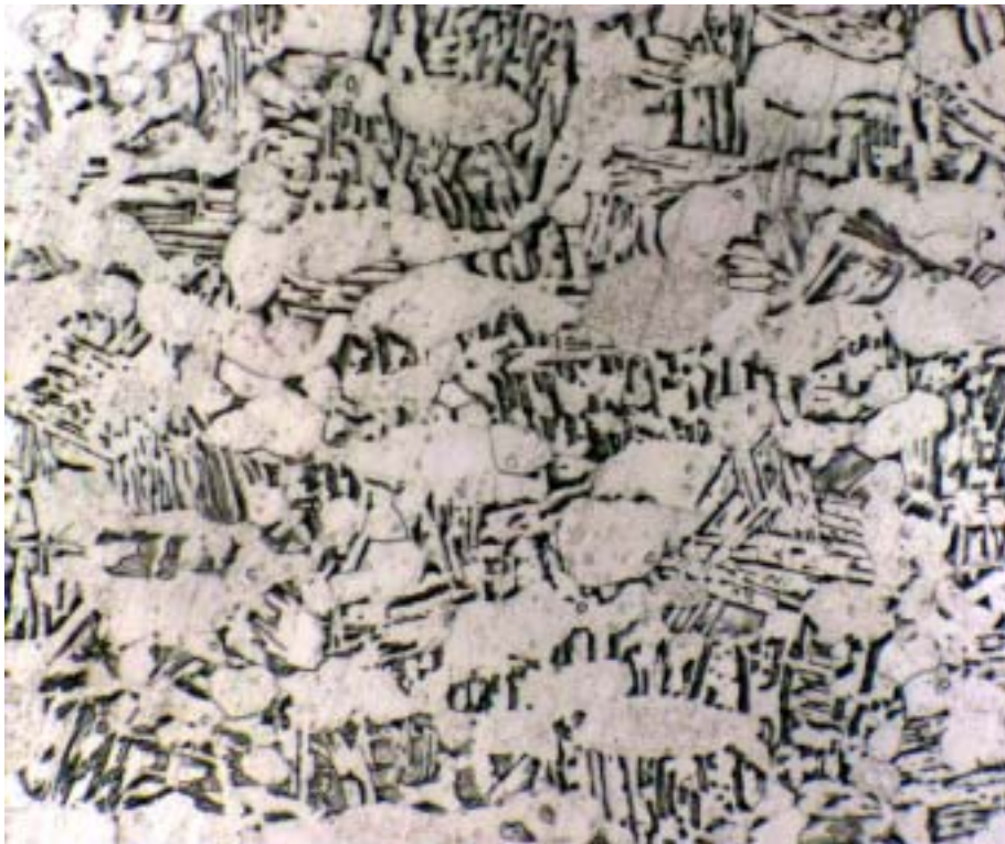
Fig. 1. Microstructure of Ti-6Al-4V alloy.
