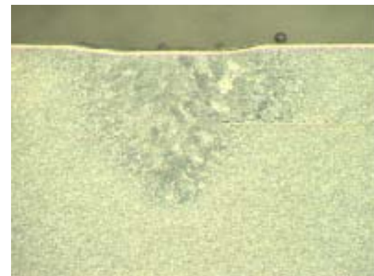
(c) 6-1 (400V, 10rpm, 7ms, 7pps)
