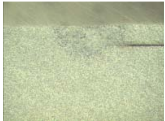
(b) 2-2 (280V, 10rpm, 7ms, 7pps)
