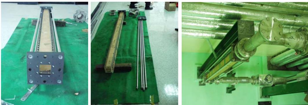
(a) Test Section Assembly, Test Section and its Support Rods
