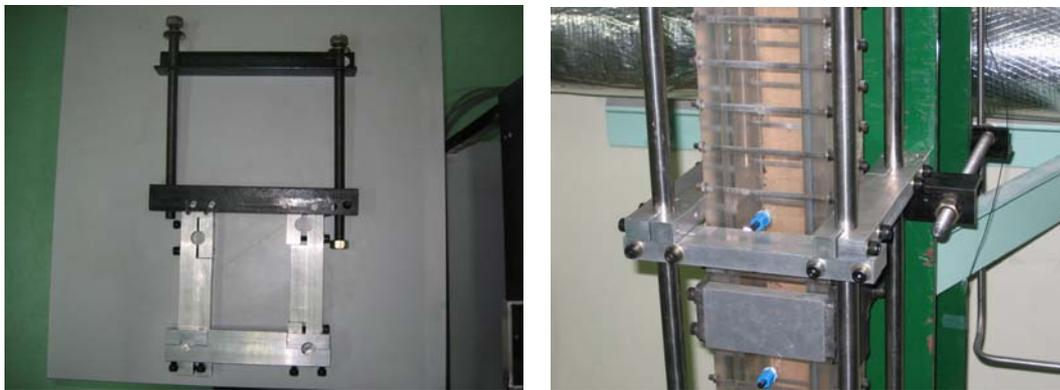
Fig. 6 Rod Clamper and Fixtures Assembly
