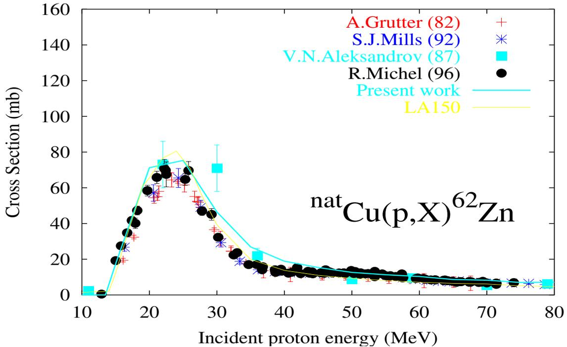
Figure 4: Evaluated  $^{nat}\text{Cu}(p,x)\text{Zn-62}$  reaction cross sections compared with experimental data and the LA150 library
