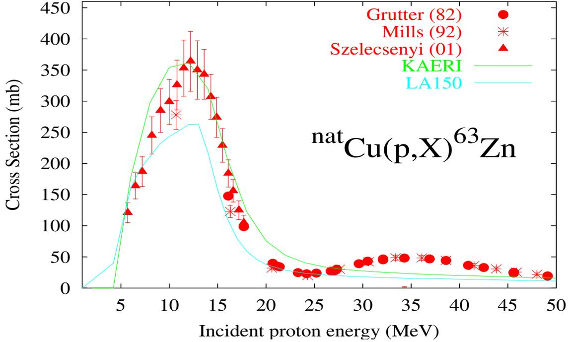
Figure 3: Evaluated  $^{nat}\text{Cu}(p,x)\text{Zn-63}$  reaction cross sections compared with experimental data and the LA150 library
