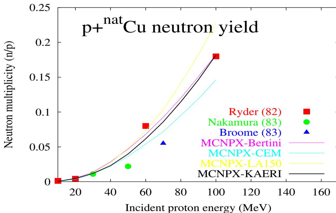
Figure 6: Number of neutrons per proton calculated in the MCNPX as a function of incident proton energies on thick copper target
