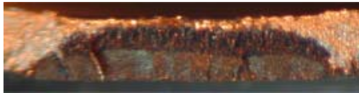
Fig. 6. Fractured surface showing the region of fatigue, ISCC and tensile rupture
