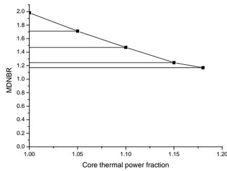
Fig. 3 MDNBR for the core thermal power
