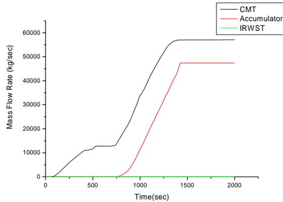
Fig. 14 Injection flow of CMT, accumulator, and IRWST
