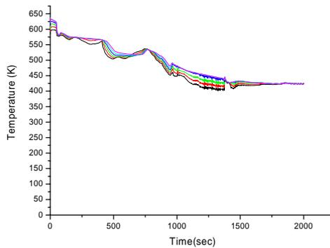
Fig. 15 Hot rod peak cladding temperature
