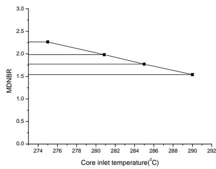
Fig. 4 MDNBR for the core inlet temperature
