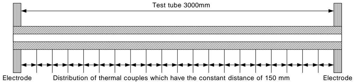
**Figure 2. Schematic diagram of test section and distribution of thermal couples along test section**
