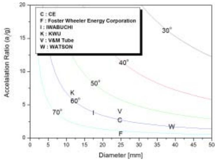
Figure 5. Acceleration ratio vs helical angle in rifled tube
