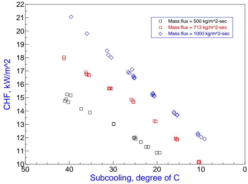
Figure 7. CHF data of R-134a at the operation pressure of 23.9 bar
