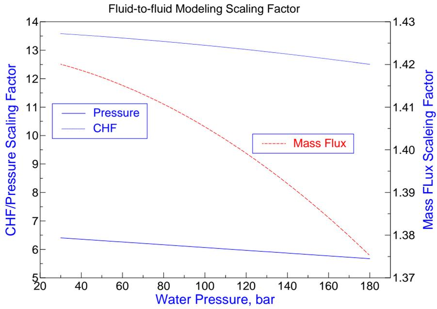
Figure 3. Scaling factors for water-to-R-134a modeling
