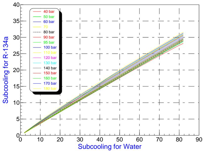
Figure 4. Relationship between subcooling degrees for water and R-134a
