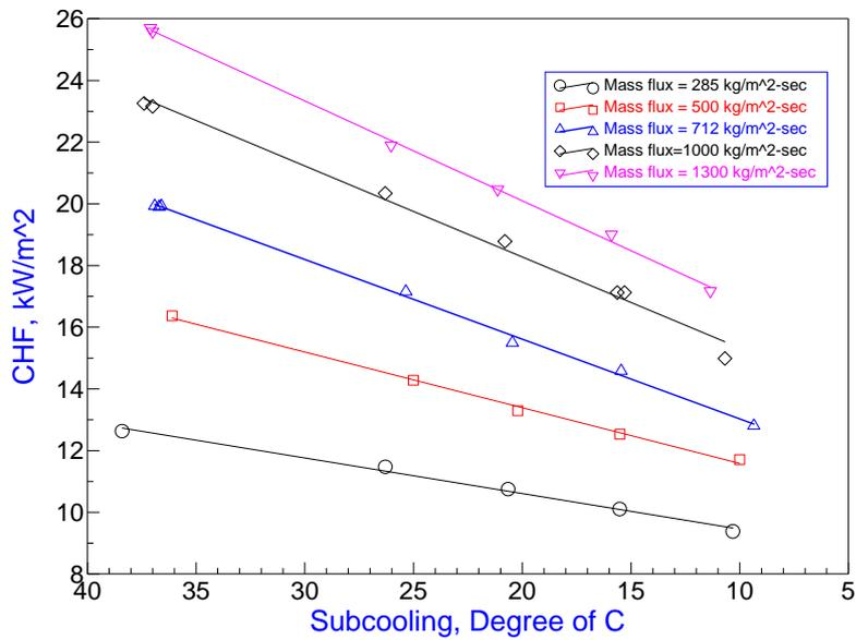
Figure 6. CHF data of R-134a at the operation pressure of 16.5 bar
