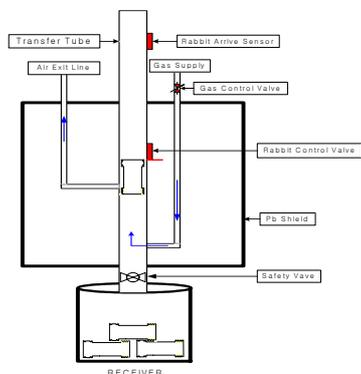
Figure 3. Schematic diagram of neutron counter column in PTS #3.
