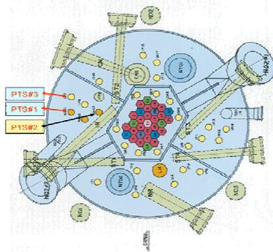
Figure 1. Irradiation sites of PTS #1 and #3 at HANARO research reactor.
