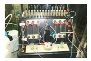
Fig. 6. [<sup>18</sup>F]FDG production module installed in hot cell, KIRAMS.
