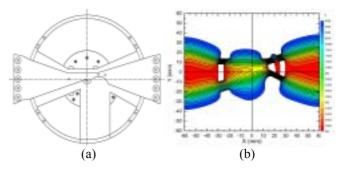
Figure 2: (a) New design of central region. (b) Electric potential map
