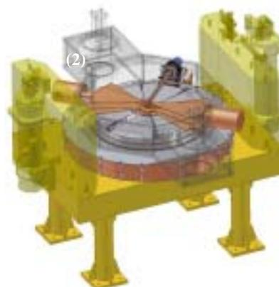
Figure. 1: Overview of KIRAMS-13. (1) Two magnetic poles, (2) A couple of Dees, (3) A PIG type ion source,
