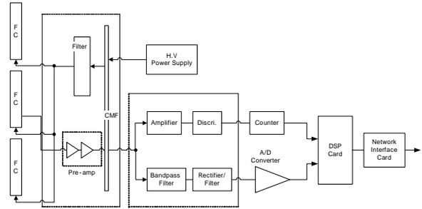
Fig 3. The simplified signal processing block diagram of Integral Reactor
