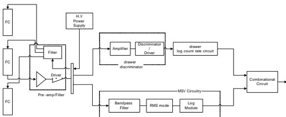
Fig 2. The simplified signal processing block diagram of built plant
