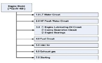
Figure 1. Subsystem of a emergency diesel generator system
