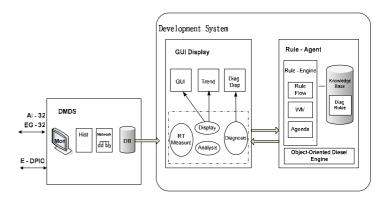
Figure 2. Structure of a monitoring-diagnosis system
