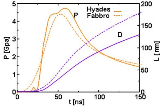
Figure 2. Comparison of Hyades simulation and Fabbro's analytical model.
