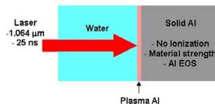
Figure 1. One dimensional model of laser produced plasma.
