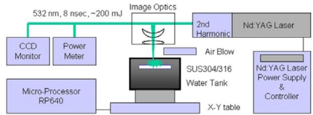
Figure 4. Schematic diagram of the Laser peening system using Q-switched Nd:YAG 2<sup>nd</sup> harmonic laser
