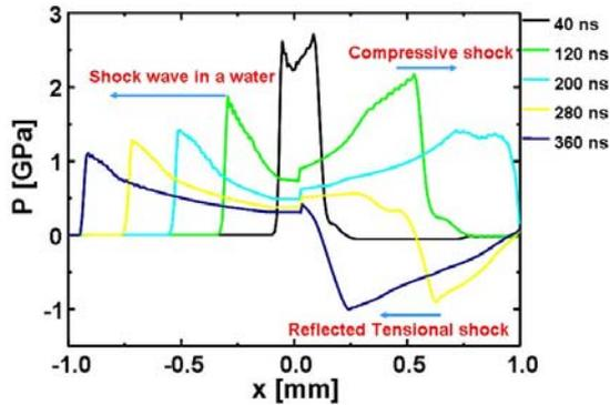
Figure 3. Shock wave propagation in metal and water.
