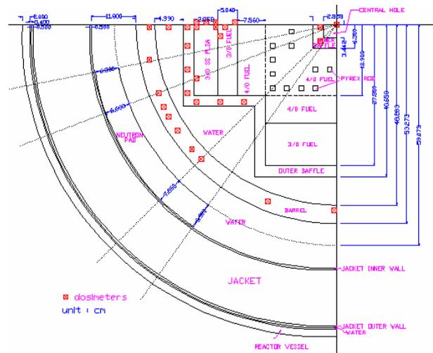
Figure 1. Cross sectional view of VENUS-3 reactor
