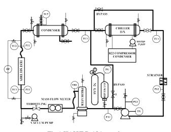
Fig.1 KAIST R-134a test loop
