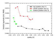
Fig. 3 Vibration Amplitude results (1000 kg/m2-s)
