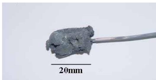
Figure 2. Photograph showing the sample cathodically treated in the Pb containing solution
