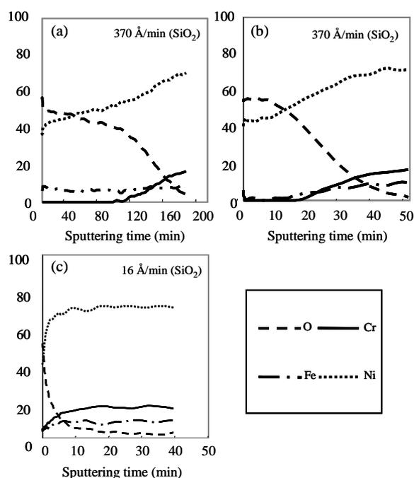
Figure 3. AES depth profiles of Alloy 600 samples exposed to 315°C, 40% NaOH solution for 4h (a) Pb-free condition without cathodic treatment, (b) Pb condition without CT, and
