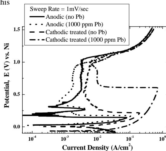
Figure 1. Polarization curves of Alloy 600 in 40% NaOH solutions with and without 1000 ppm Pb at 315°C.
