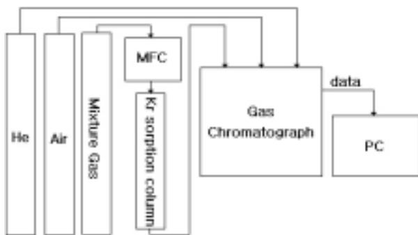
Figure 1. The Kr adsorption system and GC analyzer.
