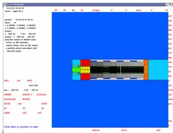
Figure 1. MCNPX Model for Accelerator Tunnel Building of KOMAC with 20 MeV Acceleration Equipments.
