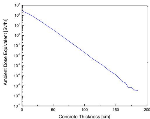
Figure 4. Dose Rate behind Concrete Shield Using Neutron Spectrum from the 20 MeV Dump
