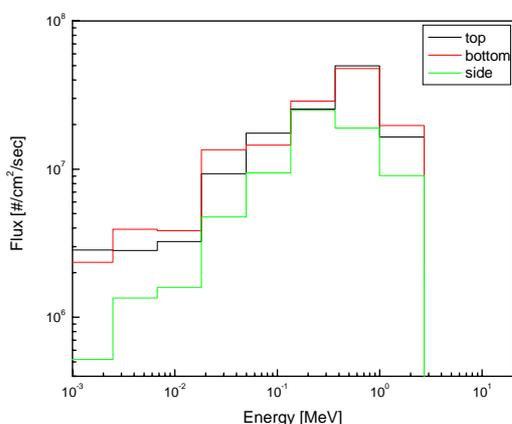
Figure 3. Neutron Spectrum from the 20 MeV Dump
