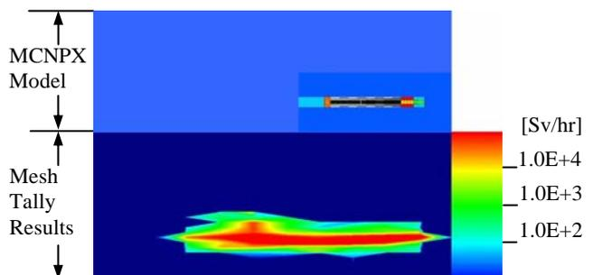
Figure 2. Ambient Dose Equivalent Distribution in the Accelerator Tunnel Building
