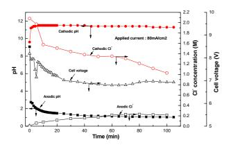
Figure 1. The changes of pH and concentrations of chloride ion in anodic and cathodic chamber of a batch electrolytic cell with circulating anolyte.
