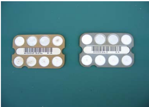
Figure 1. Exterior view of dosimeter
