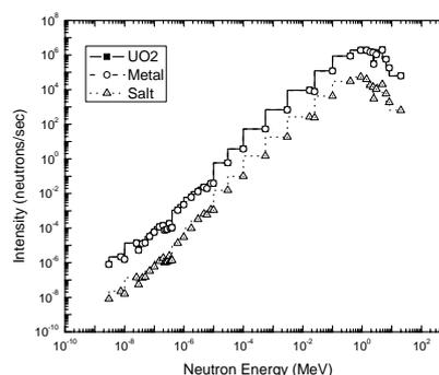
Figure 1. Neutron energy distribution of ACP materials (20kgHM basis).
