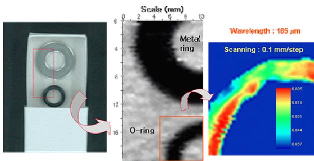
Figure 2. Transmitted THz imaging through an invisible paper box containing metal and silicon rings. We could see the shape of the rings clearly. Additionally the density information inside the silicon ring could be measured by the THz radiation.
