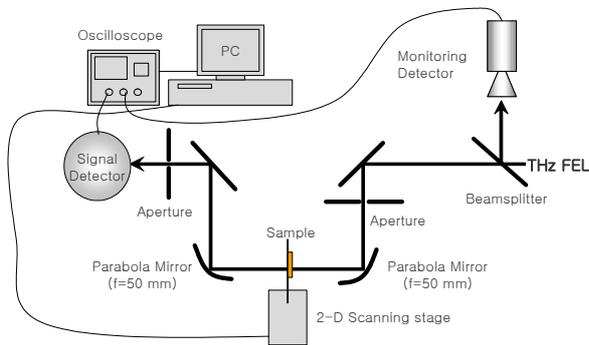
Figure 1. Schematics of the experimental setup for THz transmitted imaging with 2-D scanning of the samples.
