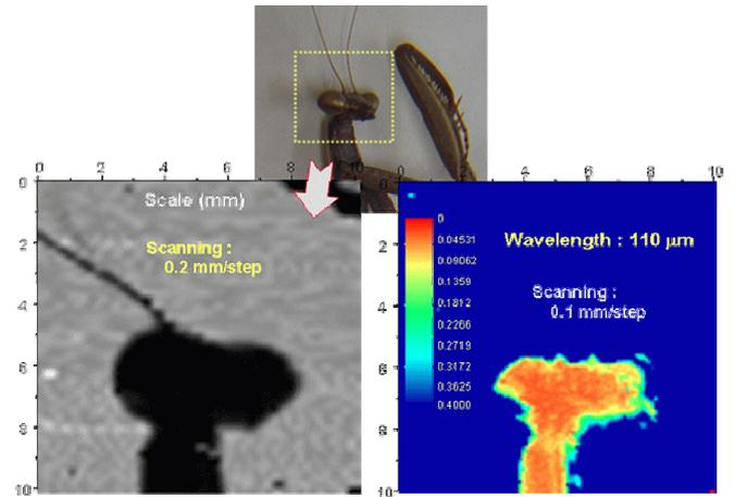
Figure 3. Transmitted THz imaging through a head part of a bug (mantis). We could see its structure information near mouse and neck part with the T-ray image.
