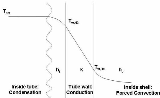
Figure 2-2 Temperature Profile in the Heat Exchanger
